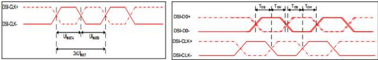
Figure 4 DSI clock channel timing
